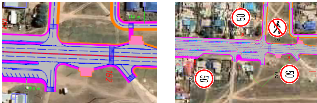
Figure 40 - Displacement of the horizontal markings of the pedestrian crossing
