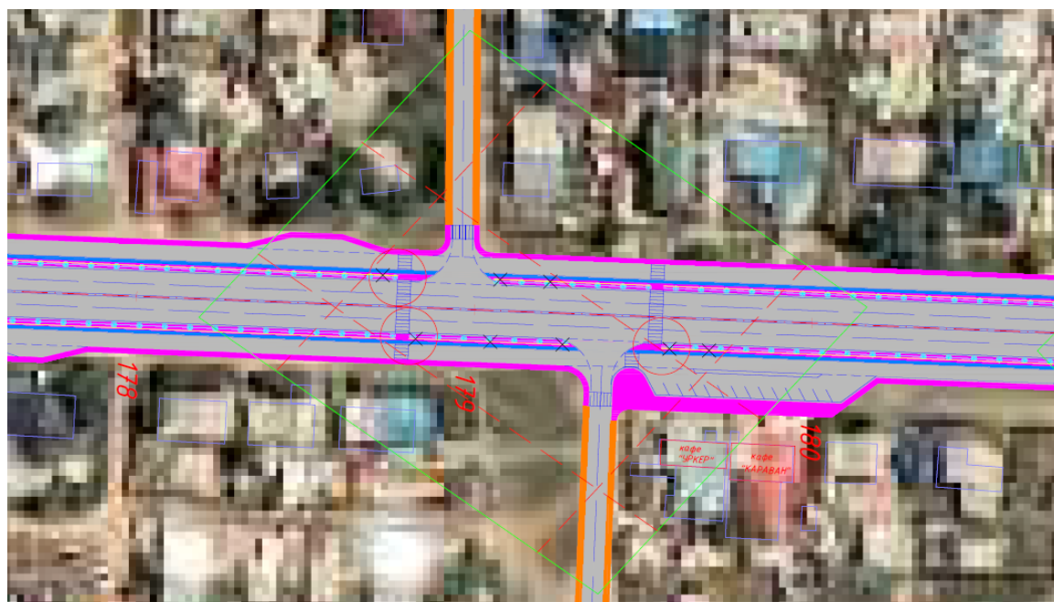
Figure 44 - Scheme of exclusion of volumes of noise barriers, with the maximum possibility of ensuring visibility at the intersection of PK178-PK179
