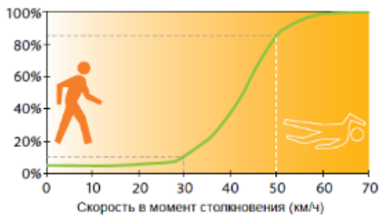
Figure 19 - Probability of death of a pedestrian in a collision with a car
